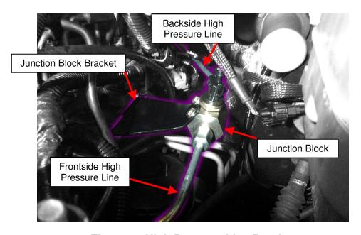
Figure 5 - High Pressure Line Routing
