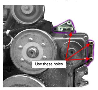
Figure 7 - Pump Support Bracket Mounting Holes
