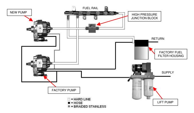
Figure 13 - Single Lift Pump System
