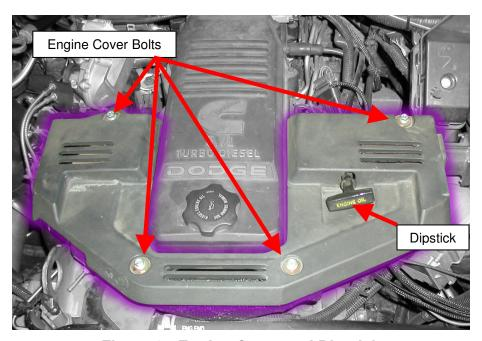
Figure 3 - Engine Cover and Dipstick
