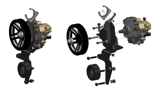
Figure 9 - Pump Mounting Assembly
