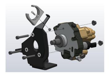
Figure 8 - Pump Bracket Assembly
