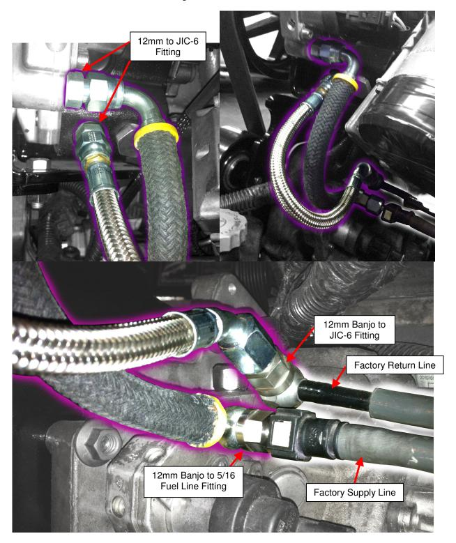
Figure 12 - Factory Lift Pump Plumbing
